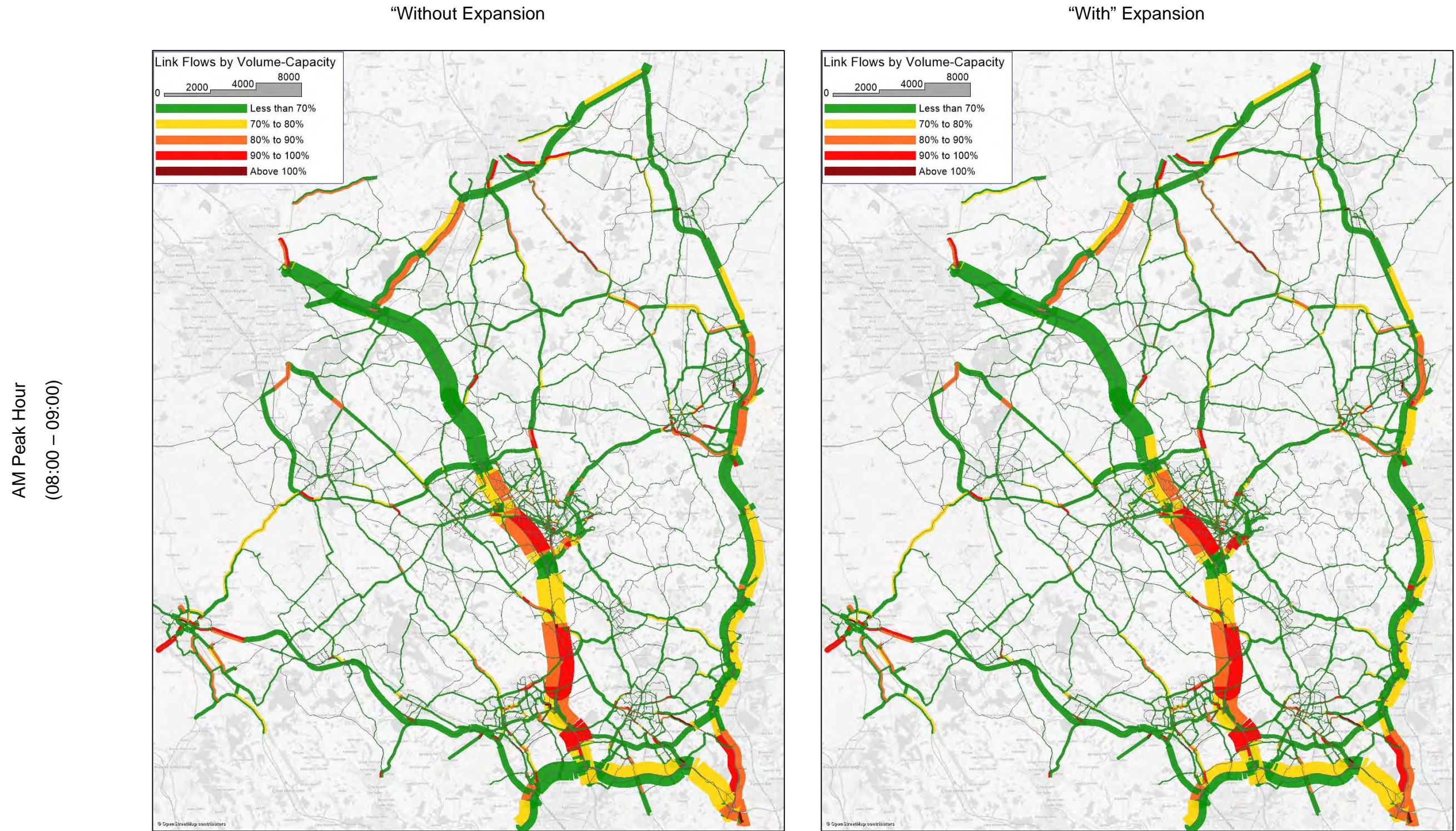
Figure F.3: Forecast Link-based V/C, Local Plan Alternative Scenario Forecasts, Simulation Network – 2043
