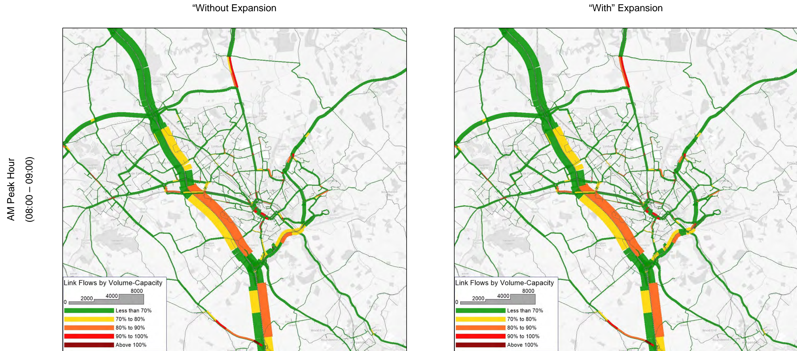
Figure E.5: Forecast Link-based V/C, TAG-based “Without” and “With” Expansion Forecasts, Luton Borough – 2027
