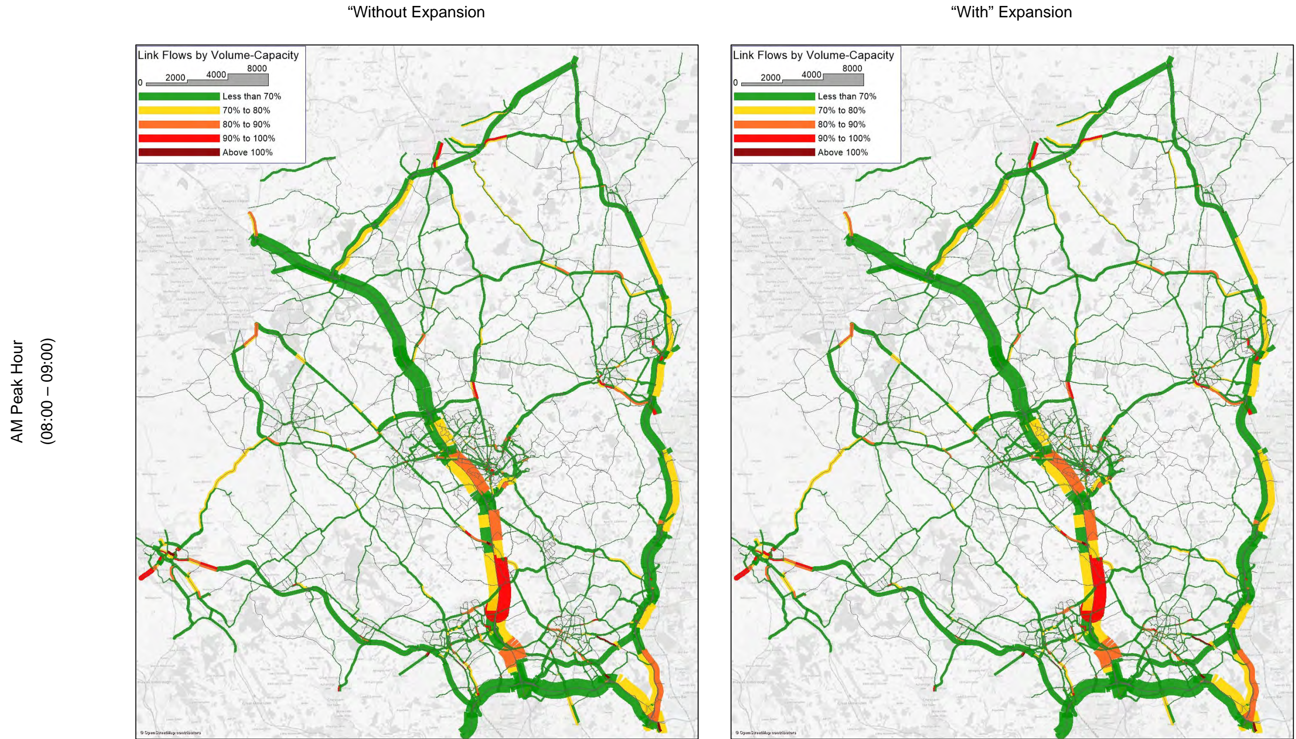
Figure E.2: Forecast Link-based V/C, TAG-based “Without” and “With” Expansion Forecasts, Simulation Network – 2027
