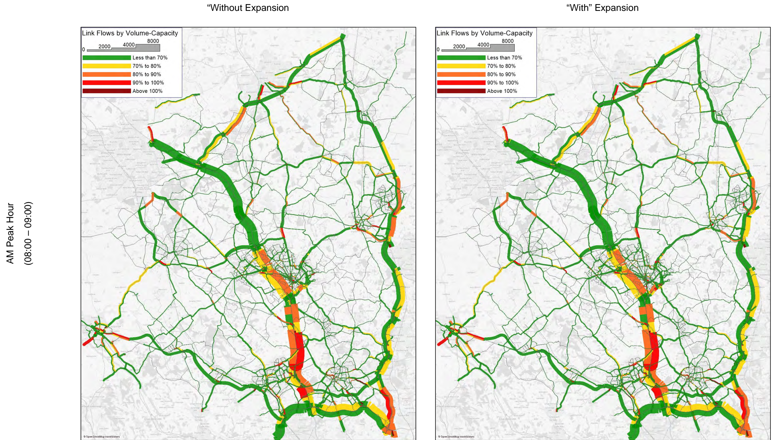
Figure E.3: Forecast Link-based V/C, TAG-based “Without” and “With” Expansion Forecasts, Simulation Network – 2039
