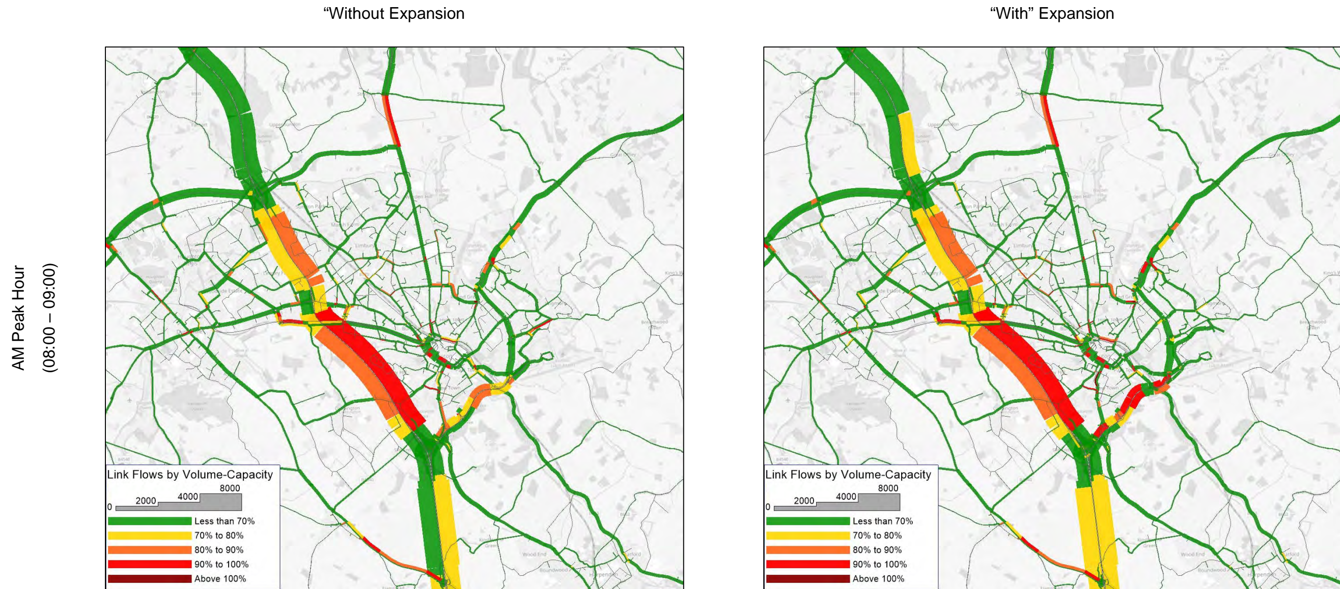
Figure E.7: Forecast Link-based V/C, TAG-based “Without” and “With” Expansion Forecasts, Luton Borough – 2043
