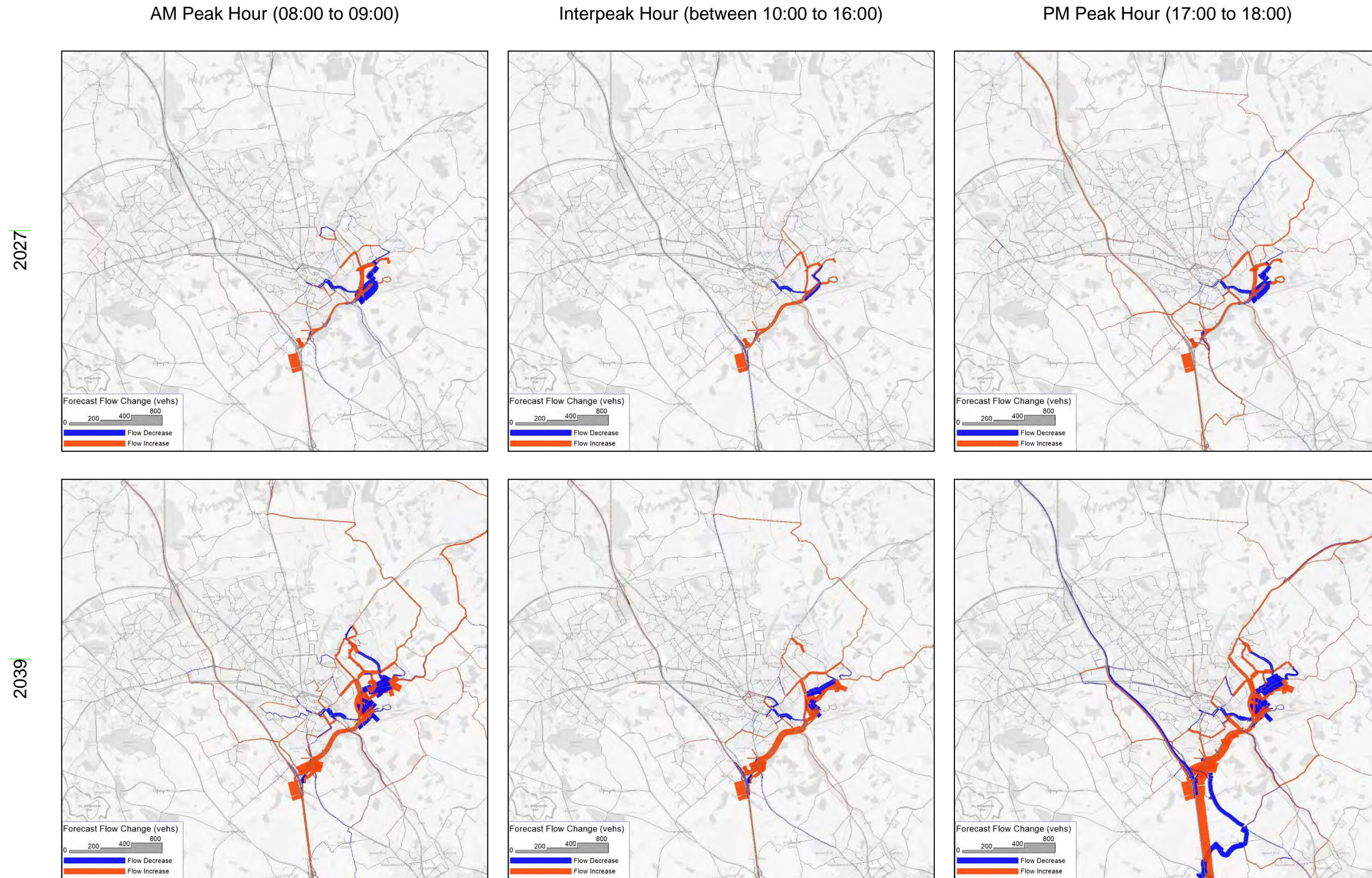
Figure 5.4: Forecast Change in Traffic Volumes (vehicles) between TAG-based “Without” and “With” Expansion, Luton Borough
