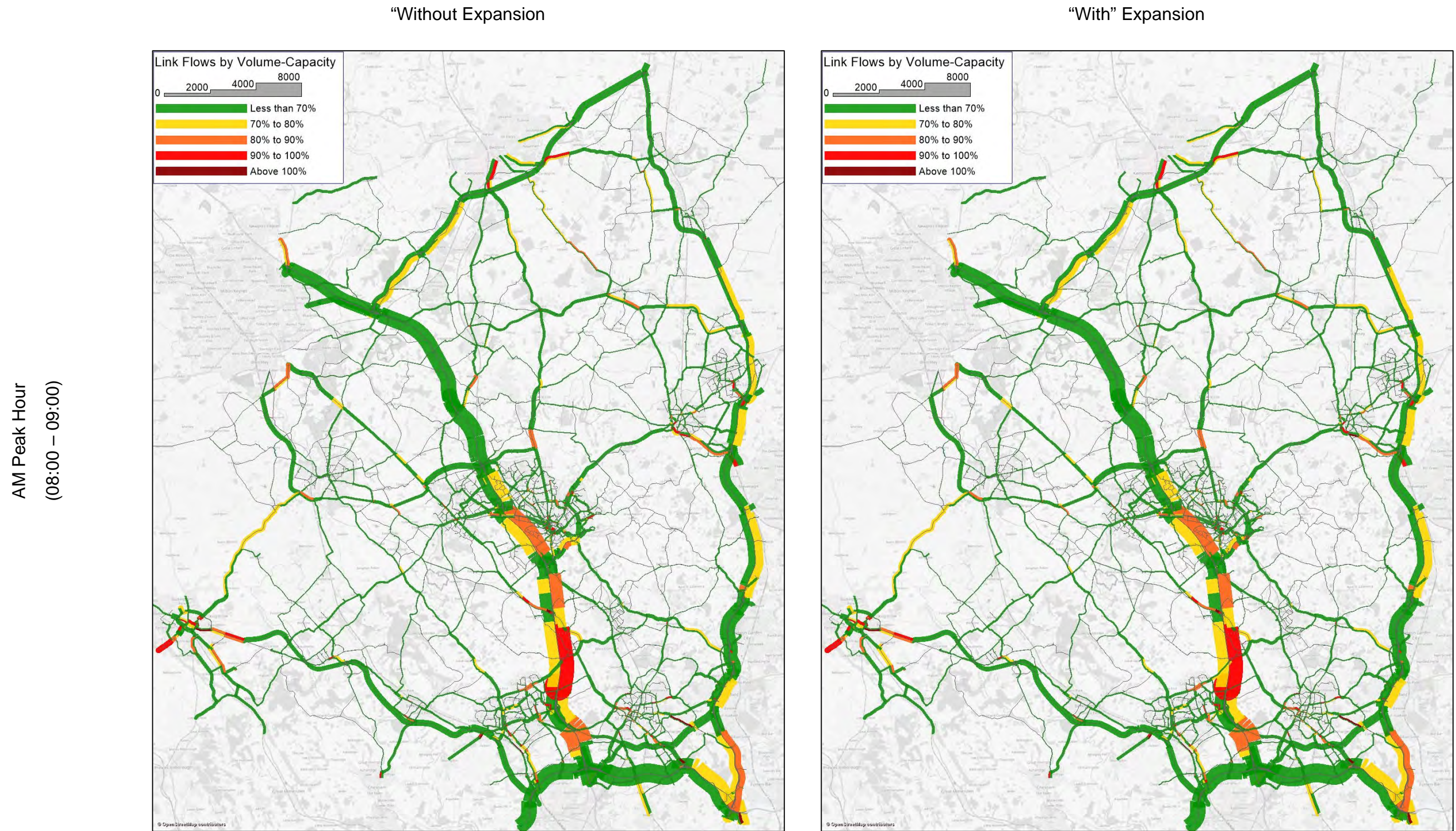
Figure F.1: Forecast Link-based V/C, Local Plan Alternative Scenario Forecasts, Simulation Network – 2027
